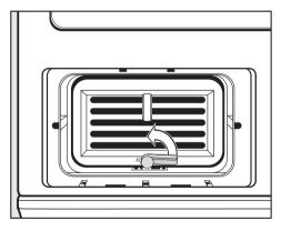
■ Turn the lever on the condenser unit to the vertical position.
